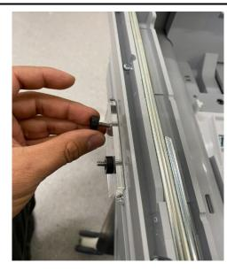
3. Mount the accessory holder and tighten the M4 nut along with the screws. Use a Phillipshead screwdriver and 7mm hex socket screwdriver as shown in the figure.
