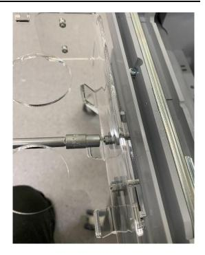
4. Check that the accessory holder doesn't make contact when the cart work-surface is slid open.
