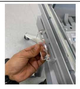
Fasten the flat clear plastic plate (1) with 2x M4x25 screws from inside the cart. Use the black plastic washers provided after inserting the screws.
